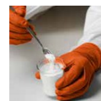
Expancel DE(T) Dry, expanded microspheres
